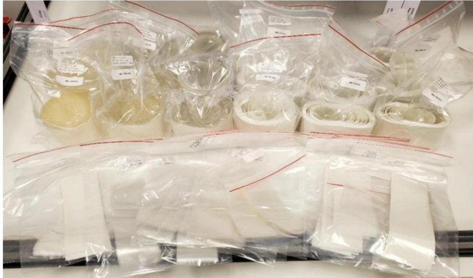
Figure 27: Test slides for setting up the NIR sorter and determining the Marker concentration for the experimental campaign
