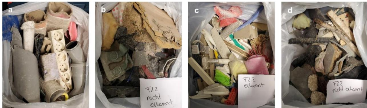
Figure 16: Sorted material from Run 1. a) F1.2, Good fractions, b) F1.2, Bad fractions, c) F2.2, Good fractions, d) F2.2 Bad fractions
