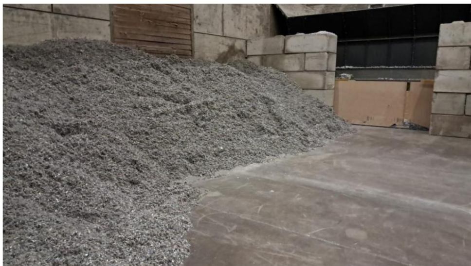
Figure 17 KORN EBS++ material after contract shredding (see Densification)
