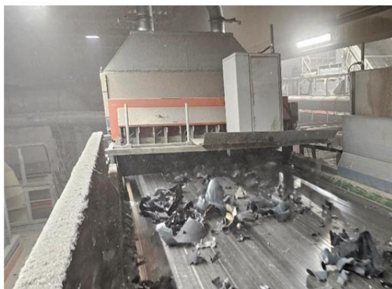
Figure 28: Sorter intended for the TBSlight trial in the KORN sorting plant
