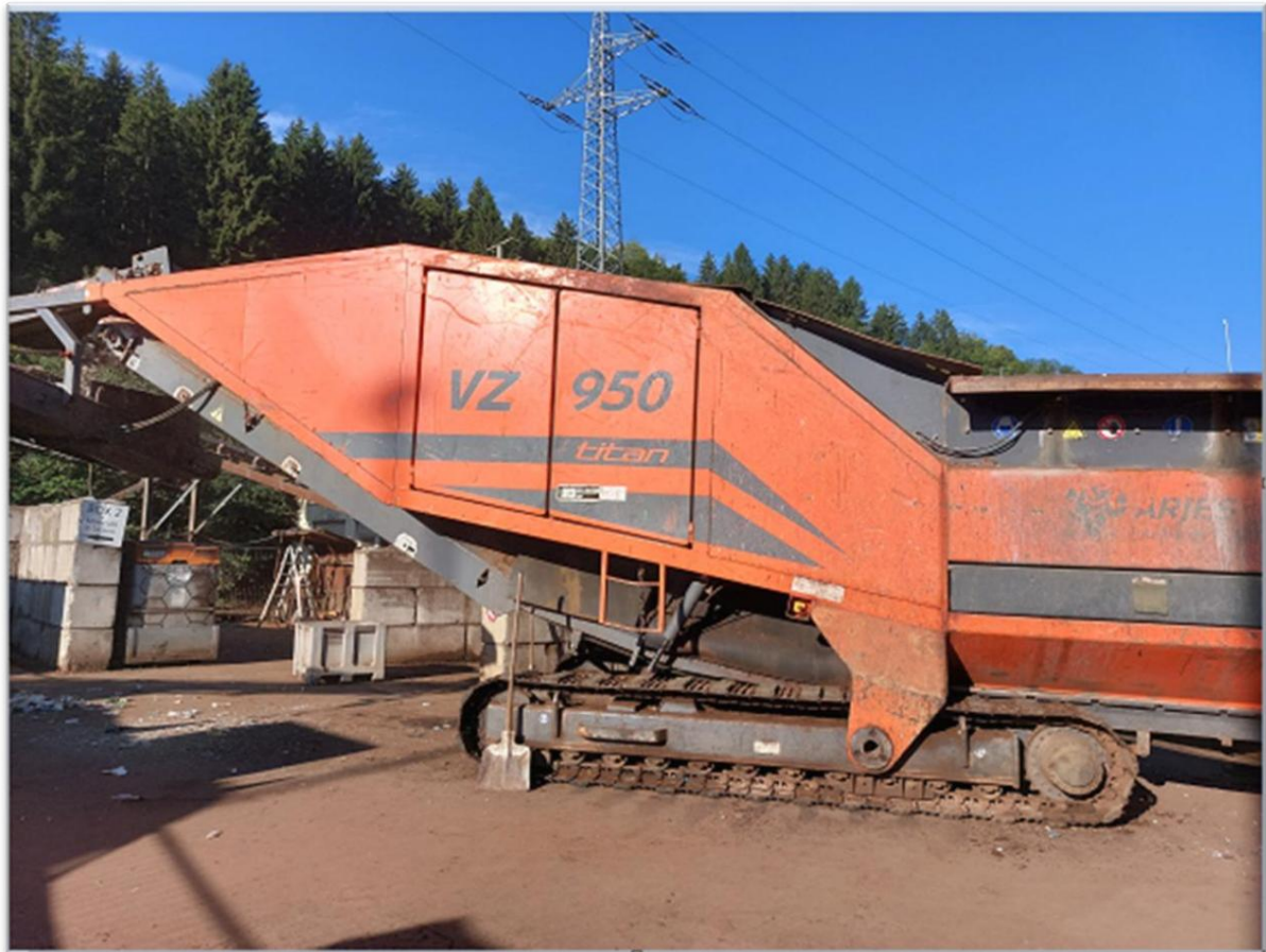
Figure 13: Mobile Arjes VZ 950 titanium re-shredder
