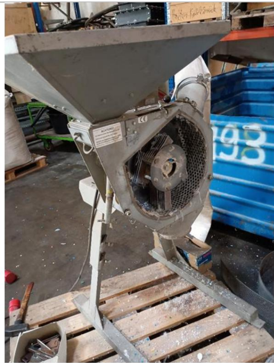
illustration 24: Cutting mill for Sample crushing in Ennigerloh
