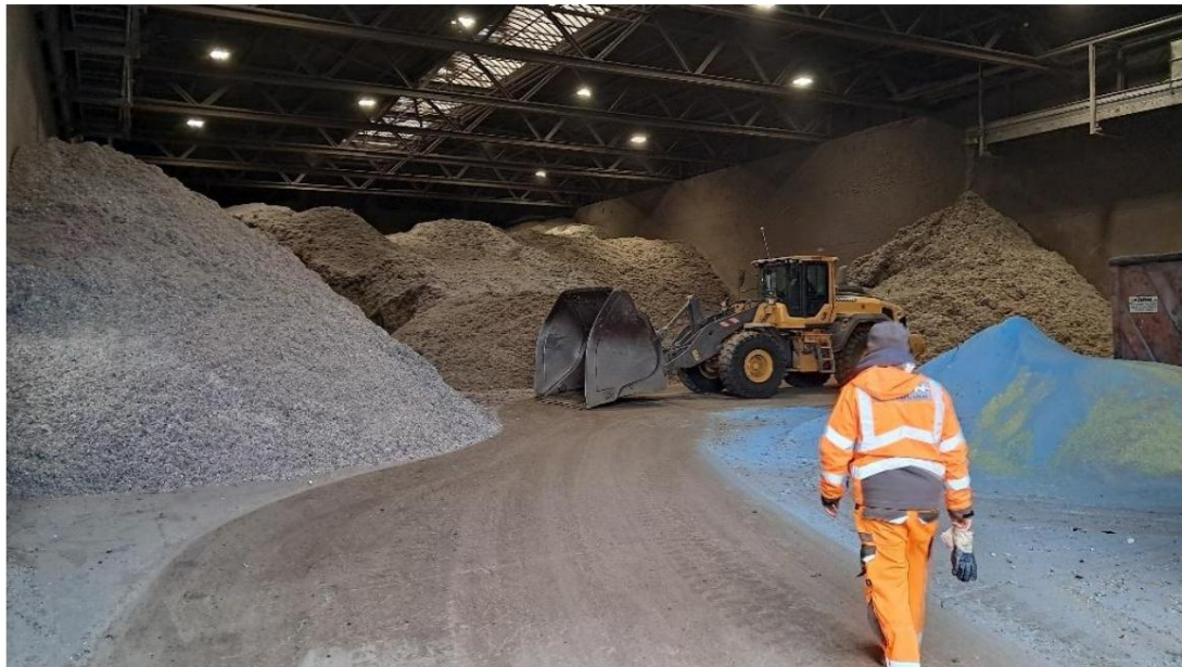
Figure 14 EBS storage facility at KORN with wheel loader for loading the truck (HN-FK-450)
