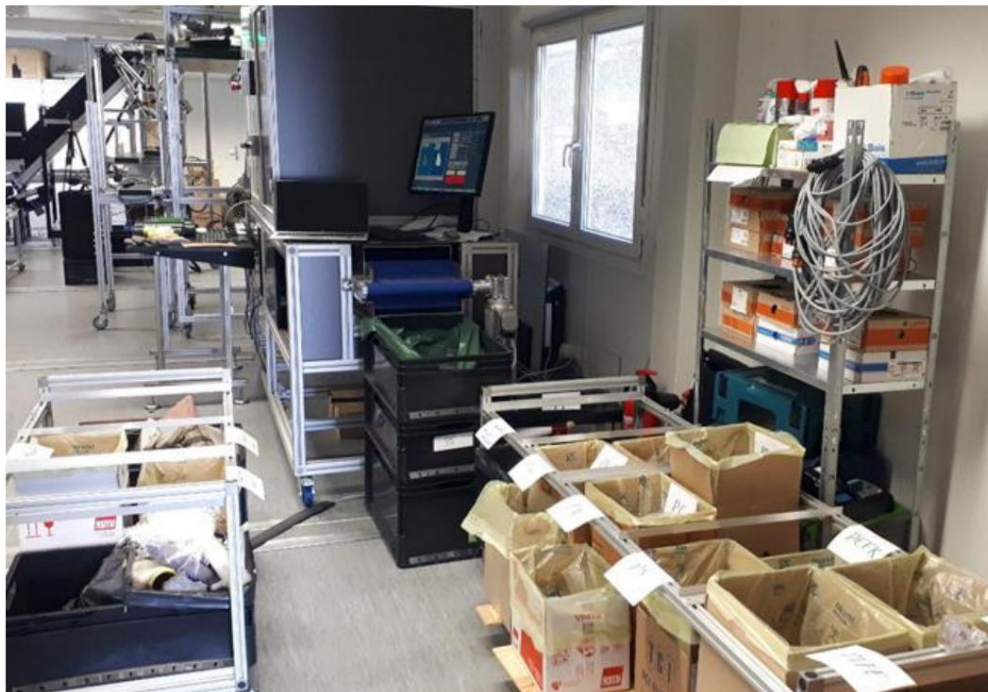
Figure 14: Setup of the storage containers for the sorting trials. In the center of the image is the end of the conveyor belt for collecting the detected parts. The parts are fed in at the opposite side.
