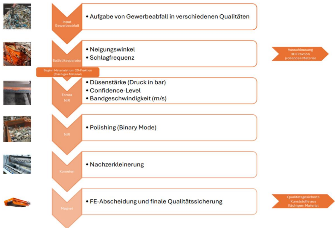
Figure 11 Process chain of the 2D fraction (series production)
